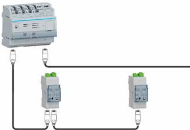
COM Modules with modbus cables
