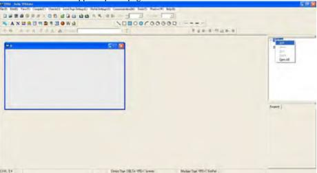
4. Download setting, Go to Tool → Communication settings (C) to set up the PC Com Port and Baud Rate. The supporting speeds of Baud rate are 9600bps, 19200bps and 38400bps. The default setting of TP address is 1, please do not modify.
