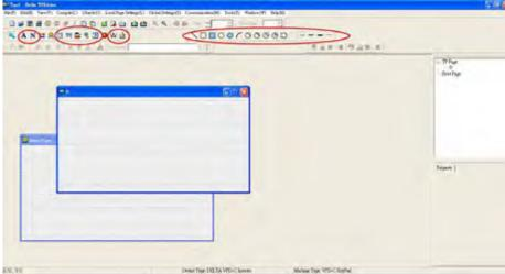
From left to right: Static Text, ASCII Display, Static Bitmap, Scale, Bar Graph, Button, Clock Display, Units, Numeric Input, 11 geometric bitmaps and different width of lines. The application of Static Text, Static Bitmap, and geometric bitmap is the same as the editing startup page.
