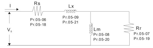
※ If Pr.05-00 is set to 2, it needs to input Pr.05-05 for motor 1/Pr.05-17 for motor 2.
