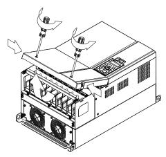
2. Remove the 5 screws shown in the following figure. Screw torque: 24~26kg-cm (20.8~22.6Ib-in).
