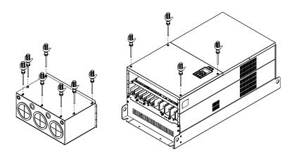
2. Remove the top cover and loosen the screws. Screw torque: 12~15kg-cm (10.4~13Ib-in).
