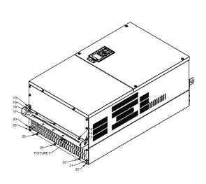
Step2. Loosen 12 screws and remove Fixture 2. Screw torque: 24~26kg-cm (20.8~22.6lb-in).
