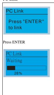
The function of PC Link is to establish a connection with computer to download the page for user defined editing. After enter to PC Link page, check if the connection of KPC-CC01 and computer is successfully establish, then press enter to go to next page and wait for communication response.
