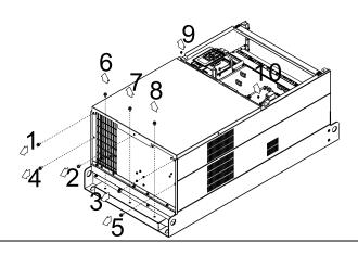
(3) Loosen screws 1~3 and remove snap bushing 4~5 (as shown in the figure below) Screw torque:  $15\sim20$ kg-cm ( $12.2\sim13.9$ Ib-in)  $_{\perp}$
