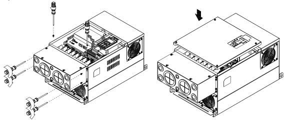
3. Fasten the 4 screws shown in the following figure. Screw torque:12~15kg-cm (10.4~13Ib-in) \_
