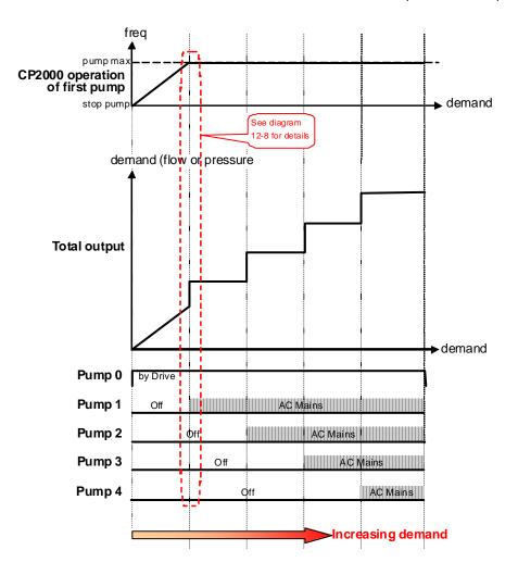
Diagram 12-8: Fixed quantity control with PID – Increasing Demand
