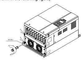
Step2. Loosen 10 screws and remove Fixture 1 (as shown in the figure below.)
