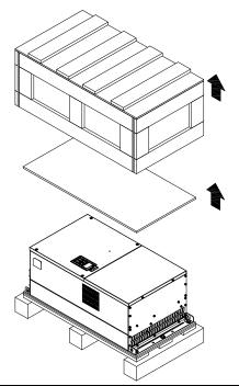
Loosen the 5 screws on the pallet as shown in the following figure.
