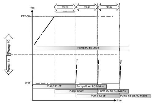
Diagram 12-9: Sequence of switching motors at Fixed quantity control with PID – Increasing Demand However, if the flow quantity or pressure is too big, CP2000 will stop, one by one, the motors from using mains electricity until CP2000 decrease the main motor's frequency to 0Hz.
