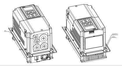
3. Plate installation, place 4 of the screw 2 (M6) through accessory 1&2 and the plate then fasten the screws. Screw torque: 25~30kg-cm (21.7~26 Ib-in) (As shown in the figures below)
