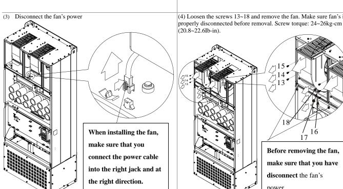
(20.8~22.6Ib-in). 13 Before removing the fan, make sure that you have disconnect the fan's power.
