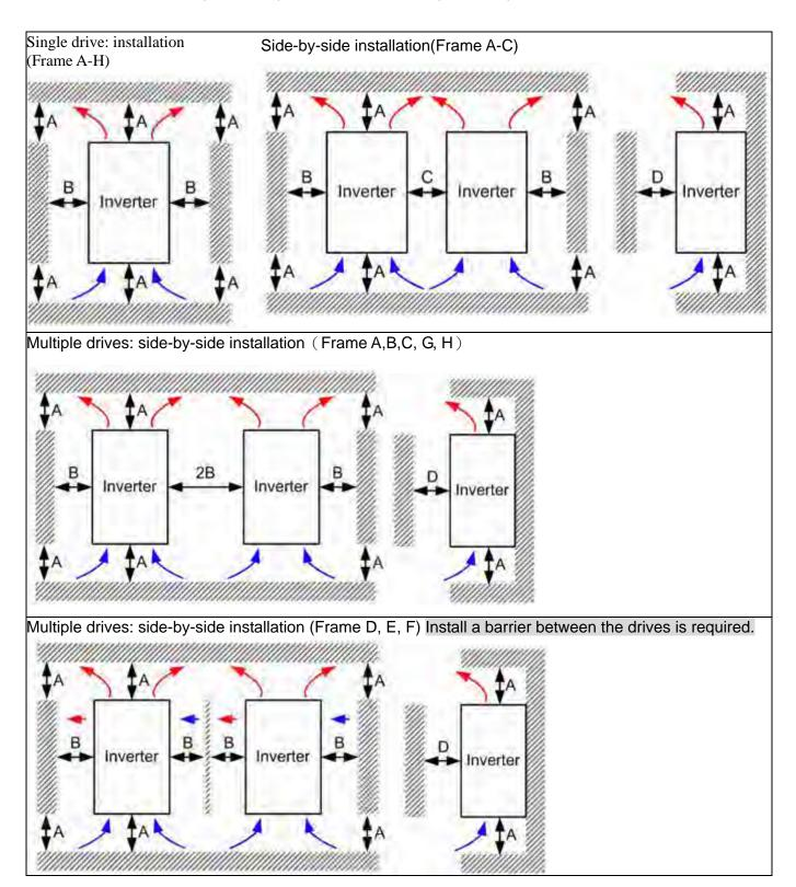
Multiple drives side-by-side installation in rows (Frame A,B,C)
