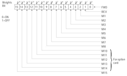
For Example: When Pr.02-52 displays 0034h(hex) and switching to 110100 (binary), it means MI1, MI3 and MI4 are used by PLC
