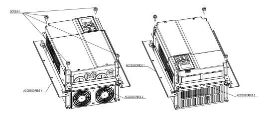
Plate installation, place 8 of the screw 2 (M6) through accessories 1&2 and the plate then fasten the screws.
