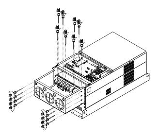
4. Fasten all the screws. Screw torque: 25~30kg-cm (20.8~30Ib-in).
