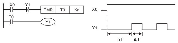
The figure above uses timer T0 to control coil Y1 to be ON. After Y1 is ON, timer T0 will be closed at the next scan period and output Y1. The oscillating circuit will be shown as above. (n is the setting of timer and it is decimal number. T is the base of timer. (clock period))
