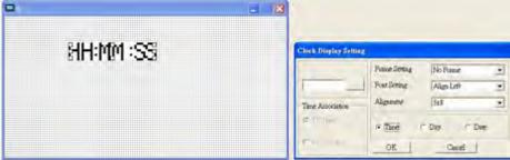
In the clock display setting, you can choose to display Time, Day or Date on the Keypad. To adjust time, go to #9 on the Keypad's menu. You can also adjust Frame Setting, Font Setting and Alignment.
