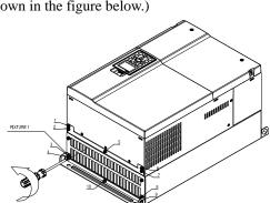
Step3. Fasten 4 screws (as shown in the figure below). Screw torque: 30~32kg-cm (26.0~27.8lb-in).
