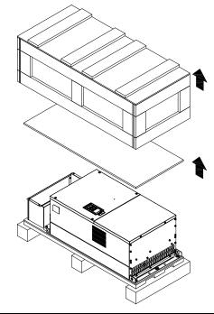
Loosen the 9 screws on the pallet and remove the wooden plate.
