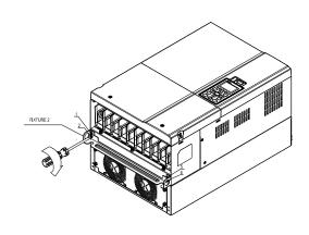
Step4. Fasten 5 screws (as shown in the figure below). Screw torque: 30~32kg-cm (26.0~27.8lb-in).
