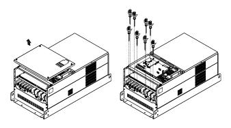
3. Install the conduit box by fastening all the screws shown in the following figure. Screw torque: 25~30kg-cm (20.8~30Ib-in); Screw torque: 12~15kg-cm (10.4~13Ib-in)
