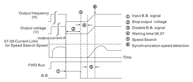
B.B. Search with minimum output frequency upward timing chart
