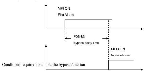
When Pr06-82 is set to 1 and under one of two conditions below.
