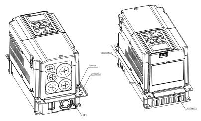
2. Install accessory 1& 2 by fastening 2 of the screw 1(M3).25~30kg-cm (21.7~26Ib-in) (As shown in the figures below)
