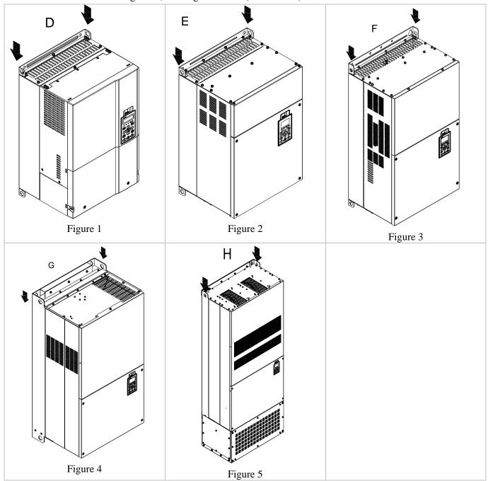
Ensure the lifting hook properly goes through the lifting hole, as shown in the following diagram.
