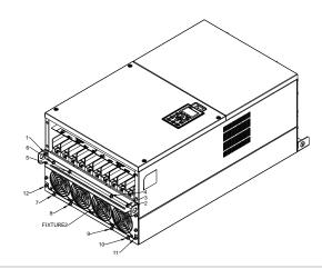
Step5. Place 4 of the M12 screws through Fixture 1&2 and plate then fasten the screws.
