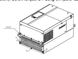
Step7. Place 4 screws (M10) through Fixture 1&2 and the plate then fasten the screws. (as shown in the following figure) Screw torque: 200~240kg-cm (173.6~208.3lb-in).
