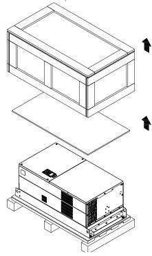
Remove the crate cover, EPEs, rubber and manual
