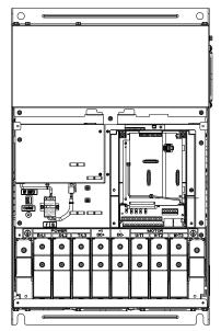
Main Circuit Terminals: R/L1, S/L2, T/L3, U/T1, V/T2, W/T3, ⊕, +1/DC+, -/DC-
