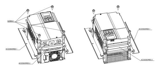
Plate installation, place 6 of the screw 2 (M6) through accessory 1&2 and the plate then fasten the screws.
