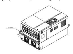
Step6. Fasten 5 screws (as shown in the figure below). Screw torque: 24~26kg-cm (20.8~22.6lb-in).
