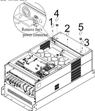
(4) Hook your index fingers to the two snap bushing holes 1~ 2(as shown in the figure below), then lift to remove the fan.
