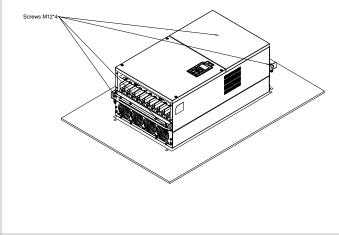
Step3. Loosen screw 13~26 and remove Fixture 1.
