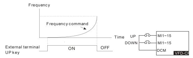
Pr.02-09 set to 1: it will increase/decrease frequency command (F) by the setting of acceleration/deceleration (Pr.01-12~01-19) and only be valid during operation.
