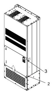
(2) Loosen the screws 5~12 and remove the top cover. Screw torque: 24~26kg-cm(20.83~22.57Ib-in)
