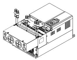
4. Fasten the 2 screws shown in the following figure. Screw torque: 10~12kg-cm (8.66~10.39Ib-in).
