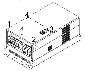
(2) Loosen the screws 1~8 (as shown in the figure below). Screw torque: 35~40kg-cm (30.4~34.7Ib-in)  $_{\parallel}$
