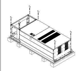
Lift the drive by hooking the lifting hole. It is now ready for installation.
