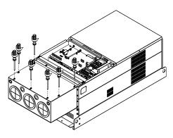
5. Place the cover back to the top and fasten the screws (as shown in the figure). Screw torque: 12~15kg-cm (10.4~13Ib-in).
