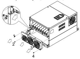
Loosen screw 1 and screw 2 (as shown in the figure below), and disconnect fan's power before removing the fan. Screw torque: 24~26kg-cm (20.8~22.6in-lbf).
