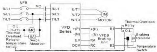
Note1: When using the AC drive with DC reactor, please refer to wiring diagram in the AC drive user manual for the wiring of terminal +(P) of Braking unit.
