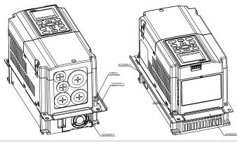
Step3. Install accessory 2&3 by fastening 2 of the screw 2(M6). Screw torque:25~30kg-cm (21.7~26 lb-in) \_
