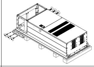
**Secure the drive from the external.** (Skip to the next step if it is not necessary in your case.)
