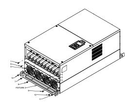
Step4. Install Fixture 1 by fasten screw 13 ~26 Screw torque: 24~26kg-cm (20.8~22.6lb-in).
