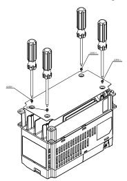
Step2. Install accessory 2&3 by fastening 2 of the screw 2(M6). Screw torque:25~30kg-cm (21.7~26.Ib-in) \_
