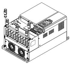
3. Install the conduit box by fasten the 5 screws shown in the following figure. Screw torque: 24~26kg-cm (20.8~22.6Ib-in).
