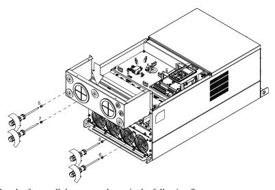
3. Install the conduit box by fasten all the screws shown in the following figure.
