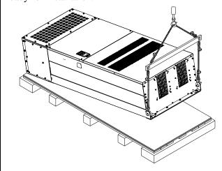
Loosen 6 of the M6 screws on the side and remove the 2 plates, as shown in below. The removed screws and plates can be used to secure the AC motor drive from the external.
