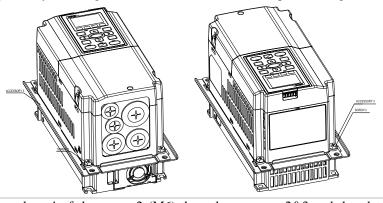
Step4. Plate installation, place 4 of the screw 2 (M6) through accessory 2&3 and the plate then fasten the screws. Screw torque: 25~30kg-cm (5.21~6.94Ib-in).25~30kg-cm (21.7~26Ib-in) \_\_
