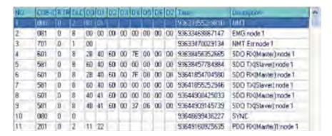
Master send NM message to slave 1 for RESET request. Slave 1 responds no error Slave 1 responds a boot up message Master enter Index6040 = 7EH in slave 1 Slave 1 responds OK Master enter Index6040= 7FH in slave 1 Slave 1 responds OK Master enter value for Index6041 to slave 1 Slave 1 responds 0640H
