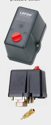
The LF18 pressure switch is used to regulate the tank pressure between two preset values on 3 phase electrically driven air compressors. It is available with an unloader valve, which prevents compressors from starting under load, and it is available with an On-Off knob for manual cut off the compressor.
