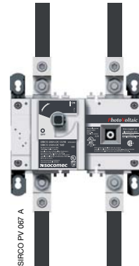
New With our new range we can break 1000 VDC with 2 poles in series.
